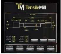
The Tensile Software also makes adding and adjusting specimen sizes extremely easy with the use of our touch screen interface. This is possible for both flat specimens on our mills and round specimens on our lathes.
